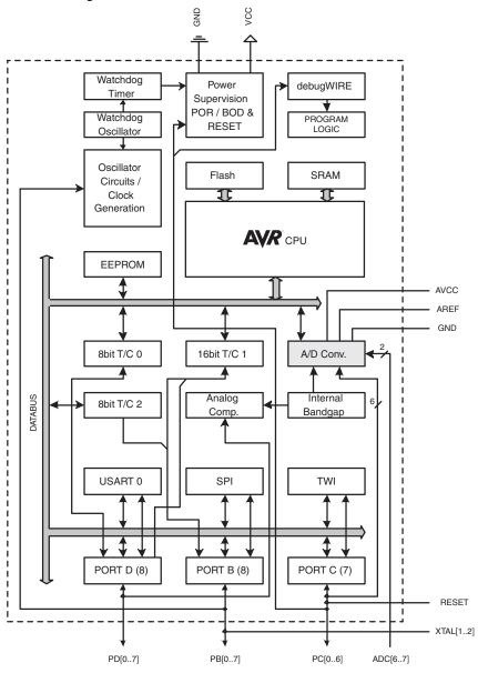
The AVR core combines a rich instruction set with 32 general purpose working registers. All the 32 registers are directly connected to the Arithmetic Logic Unit (ALU), allowing two independent registers to be accessed in one single instruction executed in one clock cycle. The resulting
