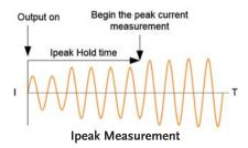
T, Ipk Hold sets delay time (1ms~60 seconds) for measurement after the output of Ipeak value and the maximum value will be retrieved. Update will be proceeded only if measured value is greater than the original value. Ipk Hold is for measuring transient inrush current as soon as the equipment power is on that is usually done by oscilloscope and current probe. T, Ipk Hold delay time setting can be applied to measure inrush current of sequentially activated DUT.
