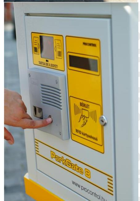
The entrance barrier opens and the driver parks the car after showing the card or pressing the button “I request a parking ticket”. The barrier does not open in the following events:
